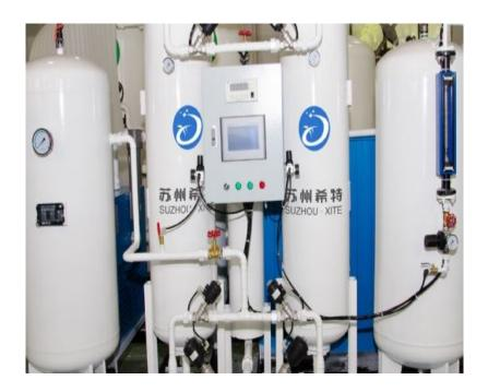
Variable Pressure Adsorption or PSA is a modern technology for on-site medical gas generators. Suzhou XITE has mastered this technology to produce the most medium to large PSA medical oxygen generators for customers in the medical industry. It can be installed in all hospitals and clinics, where patients get relief from their respiratory problems.
