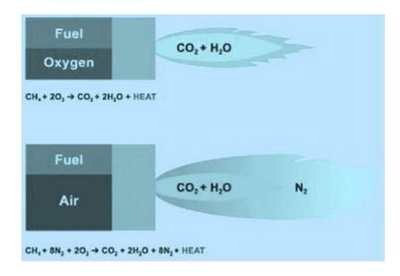
Figure 1 Oxyfuel and air-fuel combustion processes
