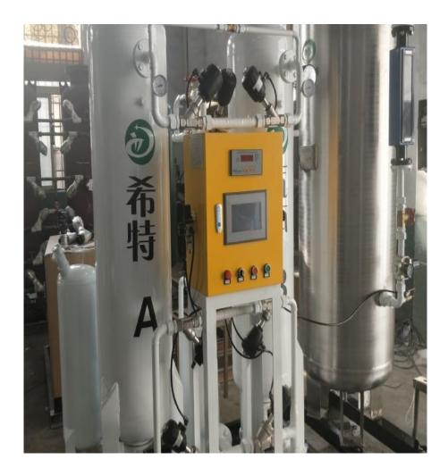
Nitrogen gases are used in various industries to create inert atmospheres. They are very helpful in generating gas at an economical price compared to liquid nitrogen/cylinder.
