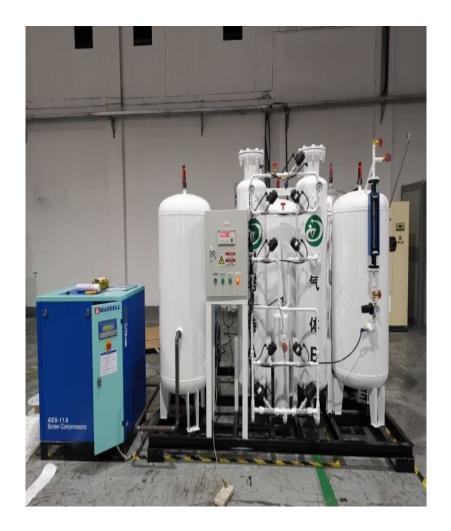
Suzhou XITE installed a 30 m3/h nitrogen generator for thermal tire cracking with 99.99% purity and 5 KG/CM2 operating pressure.
