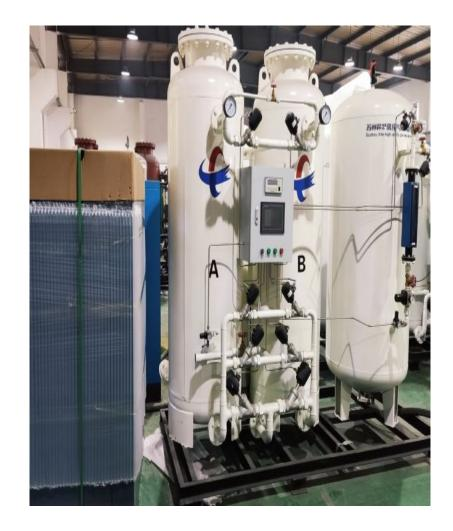
XITE supplied 2 sets of 100 m3/h nitrogen plants to a very well known manufacturer of high temperature cables.
