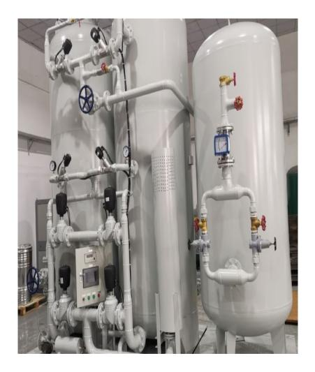
XITE installed another PSA nitrogen generator unit for our customer in Eastern China for use in the food packaging industry.
