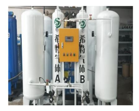
Nitrogen is used in many commercial and industrial applications to improve the quality of products or processes, or as a safety measure to prevent combustion. The delivery and storage of liquid or bottled nitrogen can be expensive, unreliable and a safety hazard. Nitrogen generators enable users to produce nitrogen simply and inexpensively in-house using existing compressed air systems.
