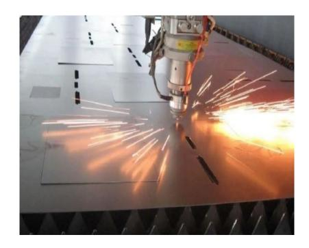
Nitrogen is an inert gas that has many uses due to its unique properties. Its inertness proves useful when driving laser cutting machines because it does not oxidize when in contact with the surrounding air. The laser beam in a nitrogen medium is also purer and more enhanced because nitrogen is a dry and clean gas.
