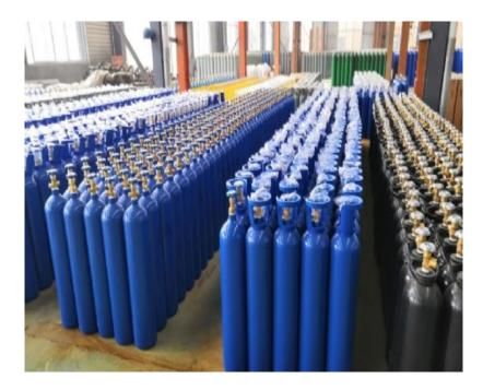
The size of a medical oxygen cylinder is measured in liters, and a 10-liter cylinder means that it can hold approximately 10 liters of water, while a 40-liter cylinder can hold 40 liters of water. The cylinder that can hold as many liters of water is called a () liter oxygen cylinder
