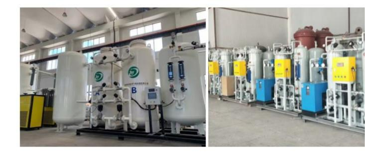
Nitrogen generator for high-purity SMT electronic assembly industry and application nitrogen generator for high-purity semiconductor industry
