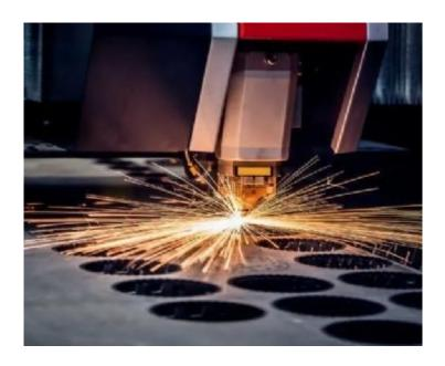
The nitrogen generator is extremely beneficial to the manufacturing business and enterprises that provide precision laser cutting services. The use of nitrogen in the laser cutting process helps to reduce the oxidation of the metal surface and provides faster and cleaner cutting.
