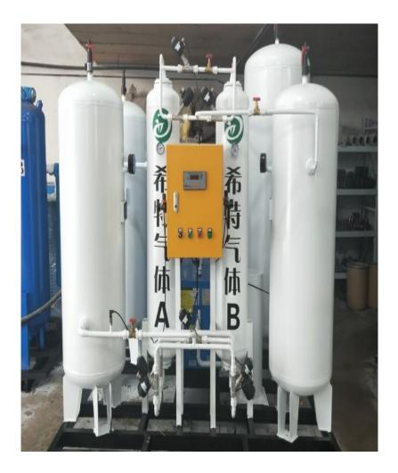
Gas Generation, Nitrogen, PSA Nitrogen Generators
