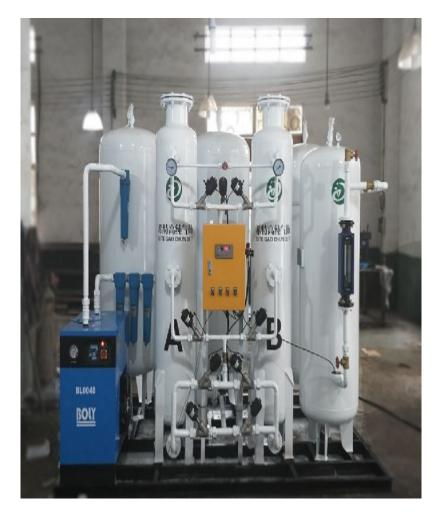
Suzhou XITE has installed a 5 cfm nitrogen generator for the oil and gas industry with 99.5% purity and 5 KG/CM2 operating pressure.
