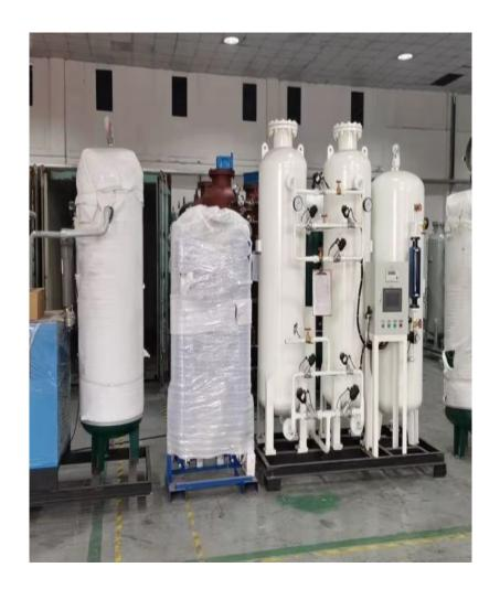
Suzhou XITE installed a 50 cfm nitrogen generator for the oil and gas industry with 99.9% purity and 5 KG/CM2 operating pressure.
