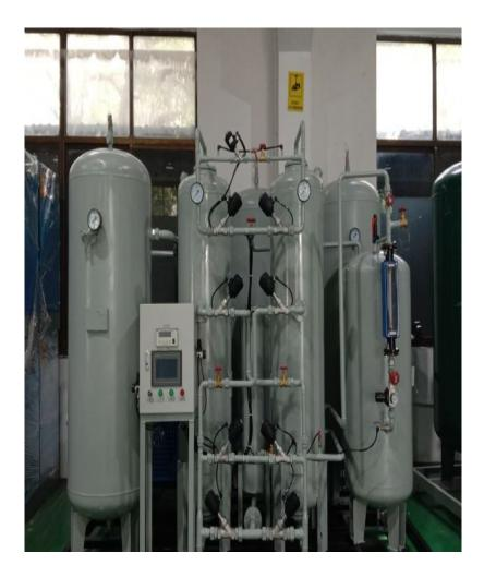
Suzhou XITE has installed a nitrogen generator for die-casting with 99.5% purity, 6 KG/CM2 working pressure and 5 cfm power.
