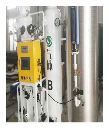
Suzhou XITE has installed a 30 cfm nitrogen generator for food packaging with 99.9% purity and 6 KG/CM2 operating pressure.
