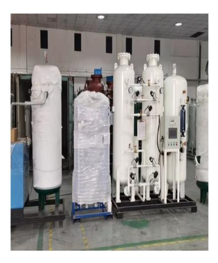
\*\*\*The company has installed a 50 NM3/HR food packaging nitrogen generator with 99.5% purity and a working pressure of 5 KG/CM2.
