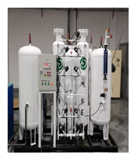
PSA Nitrogen Producer, Nitrogen Producer, Nitrogen
