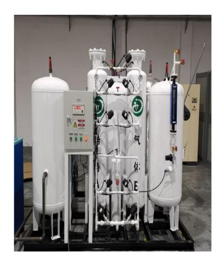
Suzhou XITE has installed a 160 m3/h nitrogen generator for food packaging with a purity of 99.5% and an operating pressure of 5 KG/CM2.
