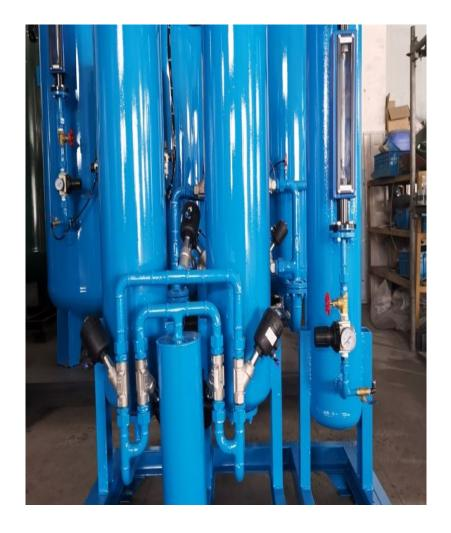
Seagate Engineering Ltd. installed a 5m3/h nitrogen generator for the annealing furnace with a purity of 99.5% and a working pressure of 5KG/CM2.
