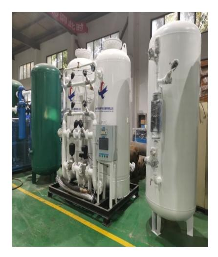
Suzhou XITE has installed a nitrogen generator for die casting with a purity of 99.9%, a working pressure of 5 KG/CM2 and a power of 30 m3/h.
