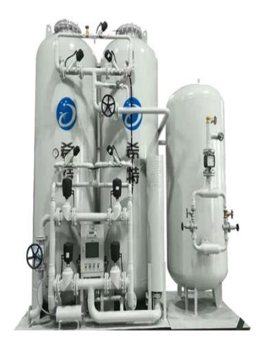
Suzhou XITE installed a 1000 m3/h nitrogen generator for thermal cracking of tires with 99.9% purity and 5 KG/CM2 operating pressure.
