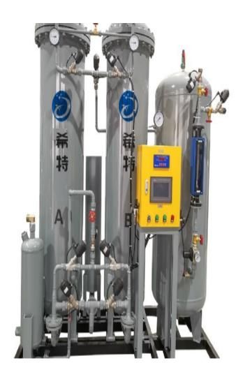
XITE Engineering Ltd. installed a 100 m3/h nitrogen generator for food packaging with 99.9% purity and 5 KG/CM2 operating pressure.
