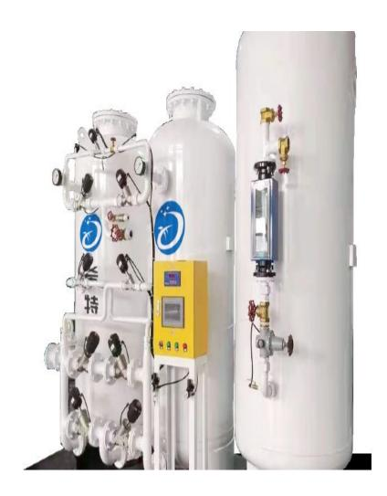
Suzhou XITE has installed a nitrogen generator for food packaging with a purity of 99.9%, a working pressure of 5 KG/CM2 and a power of 31 m3/h.
