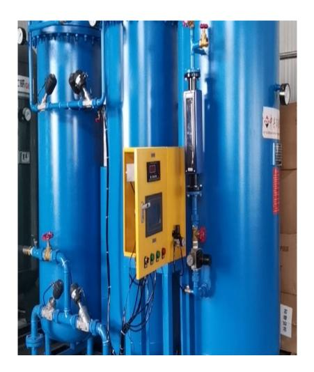
Suzhou XITE has installed nitrogen generators for food packaging with a purity of 99.50% and an operating pressure of 5 kg/cm2.
