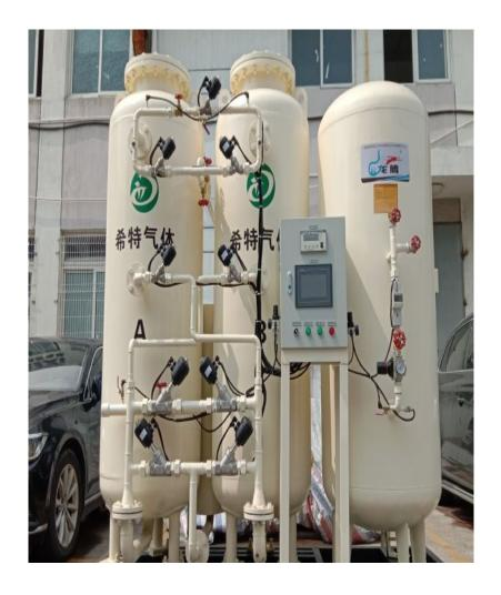
XITE Engineering Ltd. installed a 145 m3/h nitrogen generator for food packaging with 99.5% purity and 5 KG/CM2 operating pressure.
