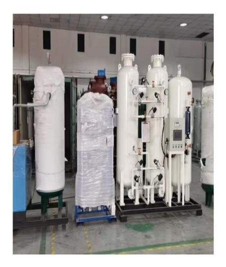
Our nitrogen generators are used in soldering processes in the electronics manufacturing industry and ensure the production of quality products in an inert atmosphere. Nitrogen helps prevent oxidation in selective soldering and convection reflow, while reflow ovens use nitrogen to provide a time and temperature controlled environment to effectively solder surface mount components.
