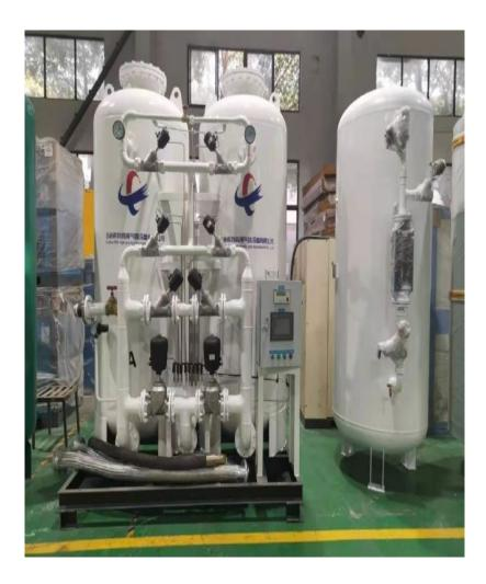
PSA or variable pressure adsorption technology is used in modern nitrogen generators, and it uses the basic principle of separating air at ambient temperature using CMS or carbon molecular sieves. If you don't know CMS, then let me explain that it is a material that adsorbs oxygen.
