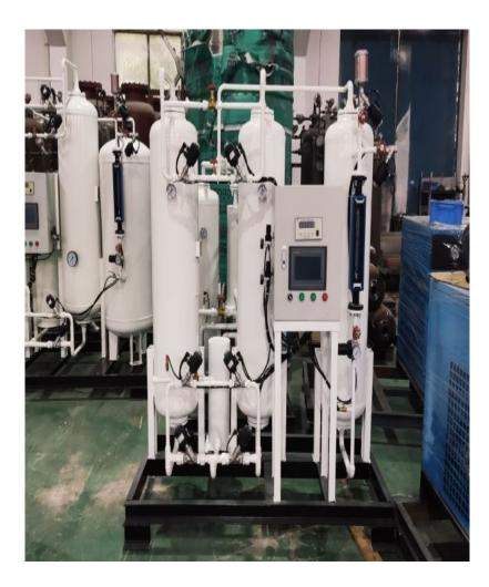
Nitrogen generators are used in a wide range of industries to provide a consistent 99.5% purity of commercially sterile nitrogen from compressed air storage tanks. For any industrial process, nitrogen generators are considered more suitable than nitrogen cylinders because the on-site equipment is more compact, reliable, and easy to use and install. However, the use of these generators is not without any risk.
